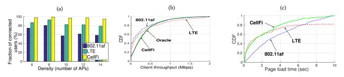
Figure 9: Coverage vs density for CellFi, Wi-Fi and LTE for 6 clients (a), client throughput of CellFi, Wi-Fi, LTE and the oracle (b), page load times of CellFi, LTE and Wi-Fi (c).
