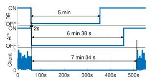
Figure 6: Spectrum database interaction experiment: At 57sec channel is removed from the DB for 5 min, 2 sec later the AP radio is turned off and the client stops transmitting.
