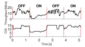
Figure 8: PHY throughput and channel quality indicator (CQI) reported during four states of interfering radio. ON denotes times where there is interference.
