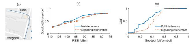
Figure 7: Outdoor LTE interference experiment setup (a), the difference between no interference and signalling-only interference (b) and the difference between signalling-only interference and data interference (c).
