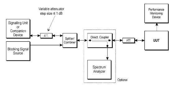
Figure 4: Test Set-up for receiver blocking
