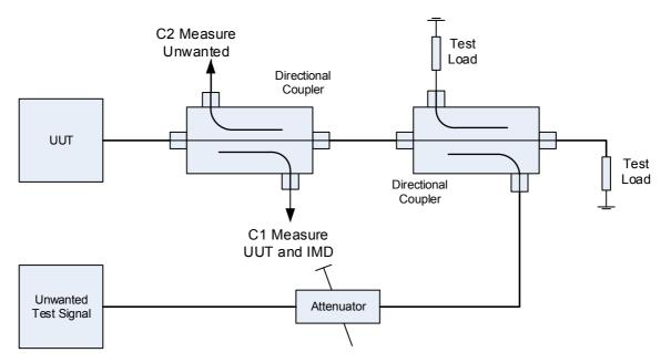
Figure 3: Transmitter Intermodulation Test Set-Up
