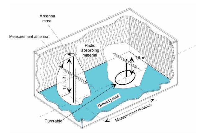
Figure B.2: A typical Semi Anechoic Room
