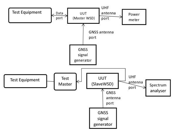
Figure 5: Test arrangement for Geo-location capability
